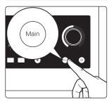
Press the Main button to enter / return to Main Output control mode. When the knob is blue it controls the main output volume.
