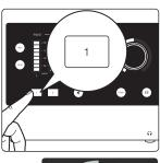
To set the gain manually, press the number of the channel that you are setting the gain for. The knob base will switch to showing relative gain level, and the knob will turn white.
