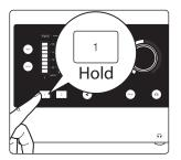
1. Press and hold the channel select button of an odd numbered channel (like 1 or 3).
