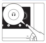
Press the headphone button to enter / return to Headphone Output control mode. When the illuminated ring around the knob is green, it controls the headphone volume.
