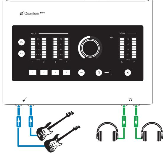
*Note:* Using the front Instrument Inputs disables the corresponding inputs on the rear panel. Unplug from the front panel to access back panel Inputs 1 & 2.
