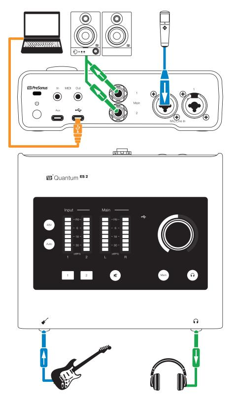
*Note:* Using the front Instrument Input disables Input 1 on the rear panel. Unplug from the front panel to access the back panel Input 1.
